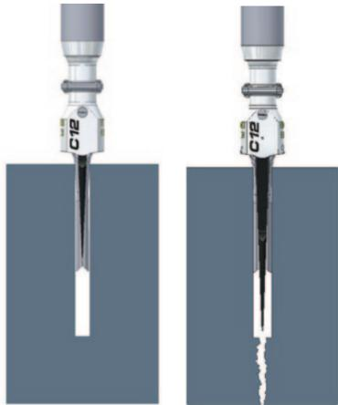
First of all, a hole is drilled to a specified diameter and depth using an ordinary rock drill. Then the wedge set is inserted into the hole with the wedge in a retraced position. The hydraulic pressure then forces the wedge between the two counter wedges, pressing them against the walls of the drilled hole. The effective splitting force of up to **413 tons** or **4048 kN** breaks concrete and rock from the inside, breaking thinner iron rods at the same time.
